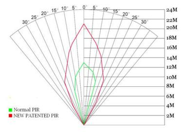
The PIR detection angle ( $\alpha$ ) is barely smaller than the field of view (FOV) angle ( $\beta$ ). This design helps reduce the empty picture rate and capture most, if not all, motions.
