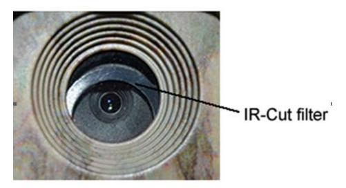
A: The camera is not broken. What's in front of the lens is called an IR-cut filter. When the camera is powered on, the IR-cut will reset and cover the lens. The IR-cut will be at a random place only when the camera is powered off.
