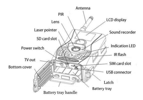
BG584 is a digital infrared surveillance camera with 4G communication functionality. It has a high sensitive Passive Infrared (PIR) motion sensor which can be triggered by any human or animal movement. The camera takes color pictures and videos at daylight and uses built-in infrared LEDs to help to take clear black&white photos or videos at night.
