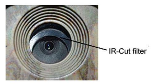
A: The camera is not broken. It's an IR-cut filter. When the camera is powered on, the IR-cut will reset and cover the lens. Only when the camera is powered off will the IR-cut be at a random place.
