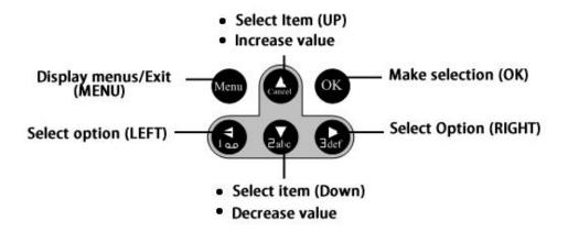
When the camera is in TEST/SETUP Mode, the screen will activate and display the following:
