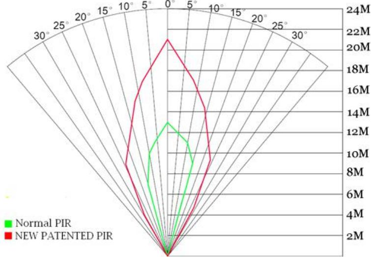
The PIR detection angle ( $\alpha$ ) is smaller than the field of view angle ( $\beta$ ). The advantage of this design is to reduce empty picture rates and capture most, if not all, motion detected.
